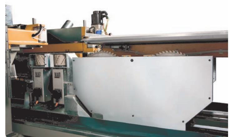
**The new working centre Fusion, which can in the meantime saw and edge-band the different elements obtained from bars.**
