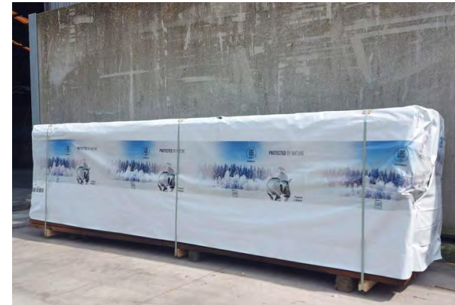
An even surface and a sufficient number of base battens prevent the products from warping.
