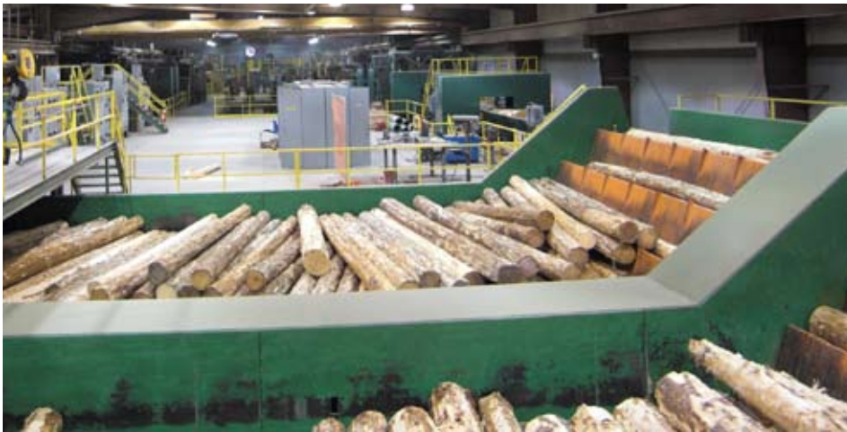
The large log line is fed by two feed modules, depending on the size of the log.
