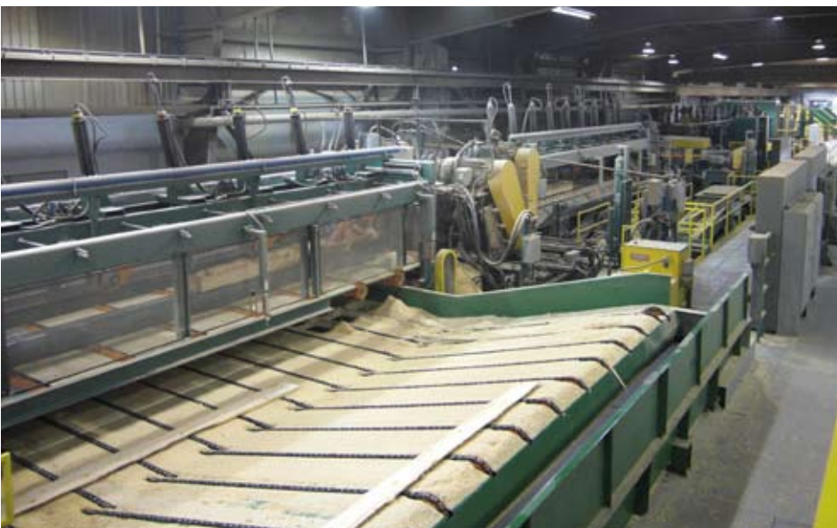
The first sawbox takes up to four sideboards off each piece, while the second sawbox, located just downstream, is capable of taking off up to six sideboards.
