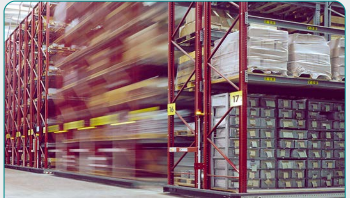
Pallet racking on carriages
