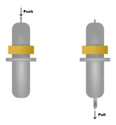
You can then remove the blade by pulling it out. Remember to replace the protective cap to ensure your blade does not get damaged or blunted.
