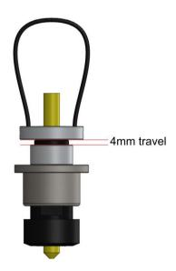
When setting the Z datum, you must position the CNC Stylus' barrel in the middle of the travel range. To do this, move your Z axis until the tool touches the material surface, and then continue to move your axis by another 2mm. You can now set your Z datum to this point.
