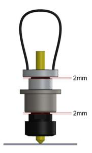
You will need to adjust the retract settings in your CAM software to ensure the CNC Stylus lifts clear of the material during a move to the start of a new toolpath. As shown, this value would need to be higher than 2mm e.g., 5mm. To learn more about retracts, and how to increase total retract height up to 19mm for special projects, please see Section 8.2 Knowledgebase, page 17.
