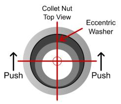
You will hear an audible click. You can check this by inverting the assembly. If the collet is fitted correctly, the collet will not fall out.
